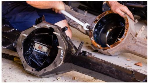
16.Replace breather from original housing. Clean internal area of new housing
